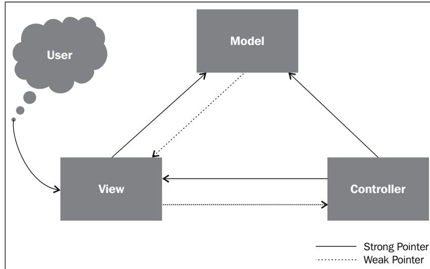
As you can see in the preceding figure, the View communicates with both the Controller and the Model. At first sight, it seems like a very flexible approach to develop an application with OOP languages. Sharing data between all objects of MVC and accessing them in any layer of application sounds very cool. Unfortunately, the method causes some problems that depend on the project's size.
