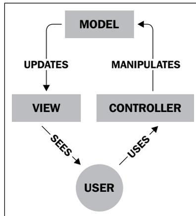
In the preceding figure, you'll see the elements of MVC. It shows the general life cycle on an MVC-based application of a request. As you can see, using an MVC architectural pattern in projects allows you to separate different layers of applications, such as the database layer and the UI layer.
