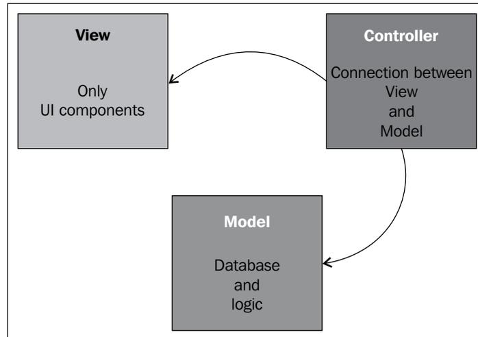
As you can see in the preceding figure, the layers of application are completely separated. Thus, you can get easily manageable code and a development team. Generally, we need at least three files in MVCs: the Model file, the Controller file, and the View file. Let's explain the View file through its objects.
