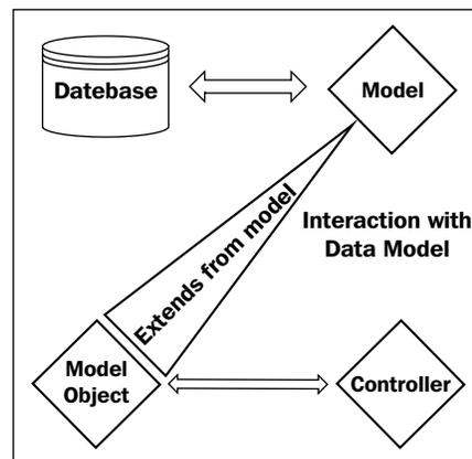
As you can see from the diagram, the Controller interacts with the Model Instance to fetch data. Since Model Instances extend from the Model itself, instead of raw Model output, the Controller can customize it or add other layers (such as Validation) to the process.
